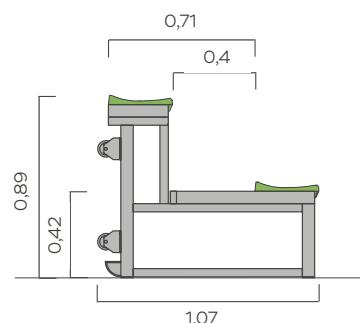
Important: the floor should not have more than 2% level variations, so that modules can be assembled together.
