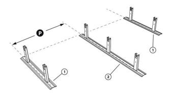
Once the rails are installed on the supports, they are fastened with screws. As the seats are already installed on their rails, they will have the distance between axes agreed for each project.
