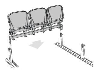
When the event for which the track seats are intended is over, the seats are dismantled following the same steps as for their installation but in reverse order. In other words, the rails are unscrewed to mount them on their trolleys, and then the supports are also stored on the corresponding trolleys.
